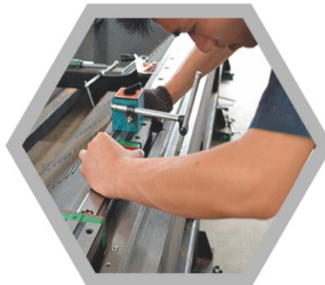
Parallelism Ball gear parallelism test
