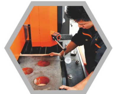
Perpendicularity Marble feet for lathe bed verticality test
