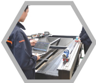
Straightness Laser collimator detects guide line
